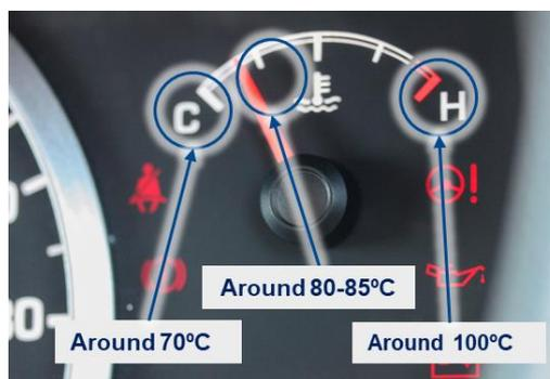
Figure 9 – Water Temperature Gauge
