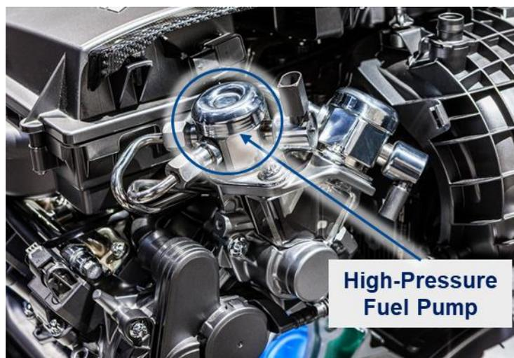
Figure 7 – High-Pressure Fuel Pump Position
