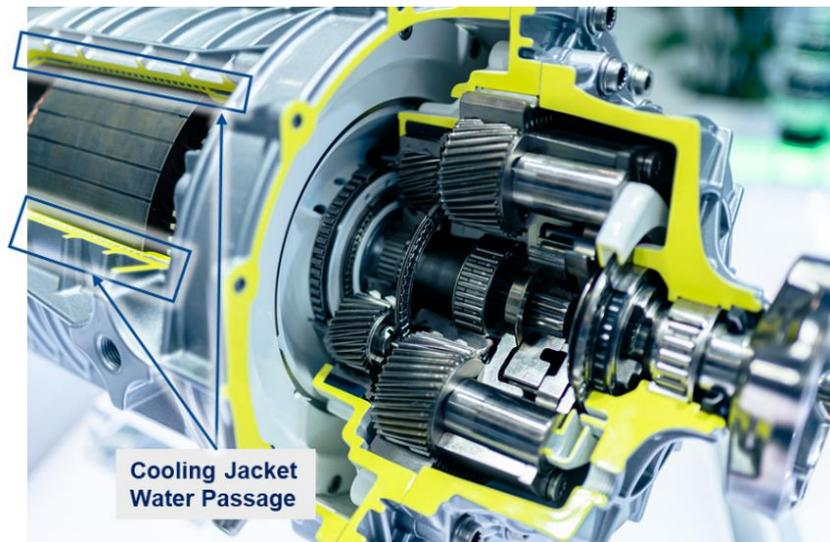
Figure 14 – Cooling Jacket Cutaway Section
