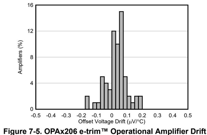
**Figure 7-5. OPAx206 e-trim™ Operational Amplifier Drift**
