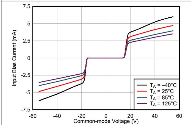
Figure 5-21. Input Bias vs Overvoltage-Protected Common-Mode Range
