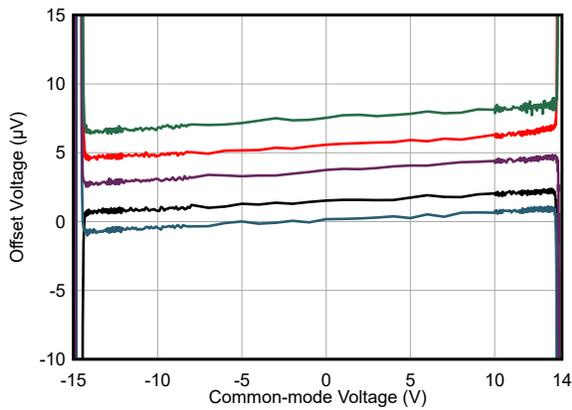
**Figure 5-11. Offset Voltage vs Common-Mode Voltage**
