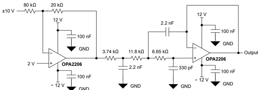
**Figure 8-1. OPA2206 Configured as a Voltage Attenuator**
