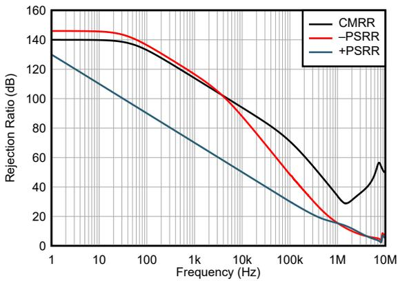
**Figure 5-9. Power-Supply and Common-Mode Rejection Ratio vs Frequency**
