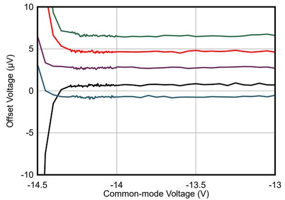
**Figure 5-12. Offset Voltage vs  $V_{CM}$  at Low Supply**
