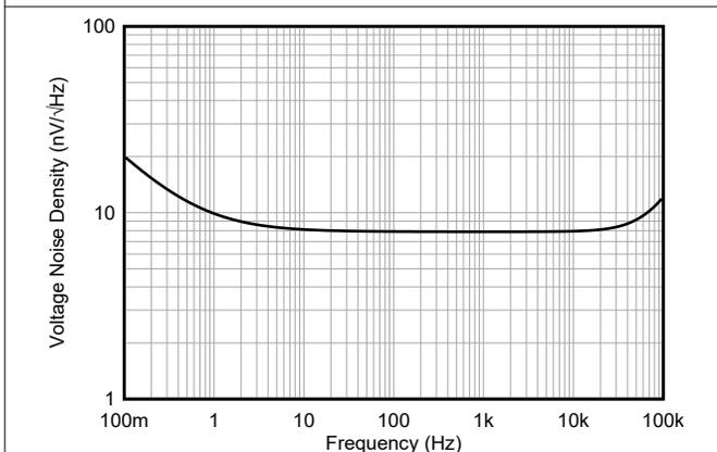
Figure 5-23. Voltage Noise Density vs Frequency
