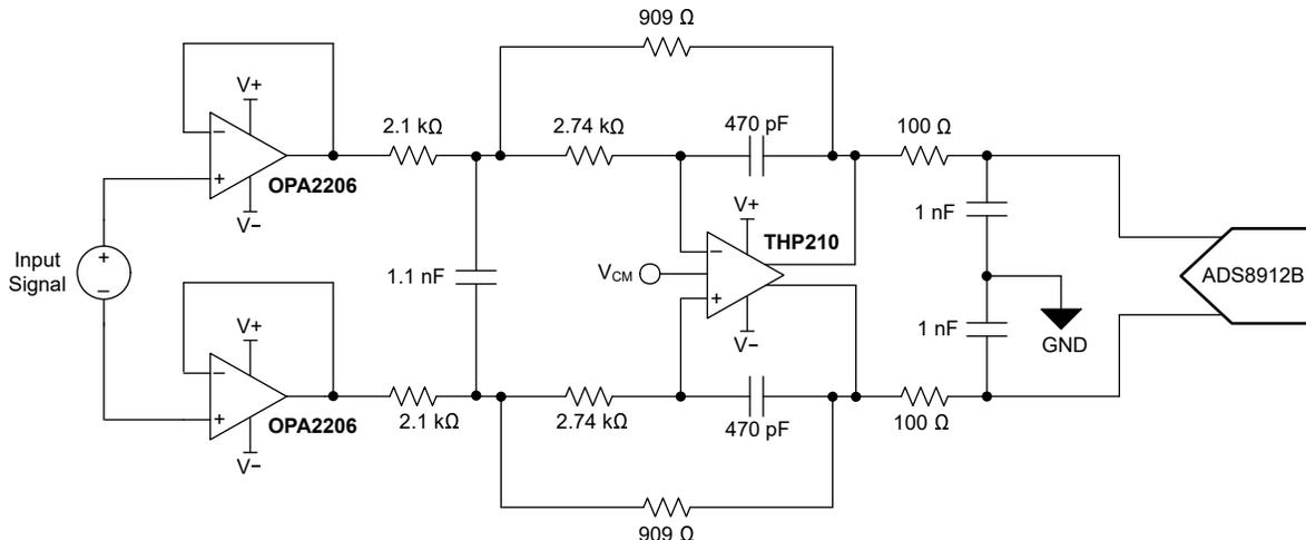
Figure 8-5. OPA2206 Configured as an Input-Signal-Chain Buffer
