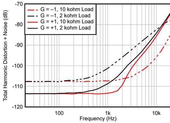
**Figure 5-25. Total Harmonic Distortion + Noise Ratio vs Frequency**
