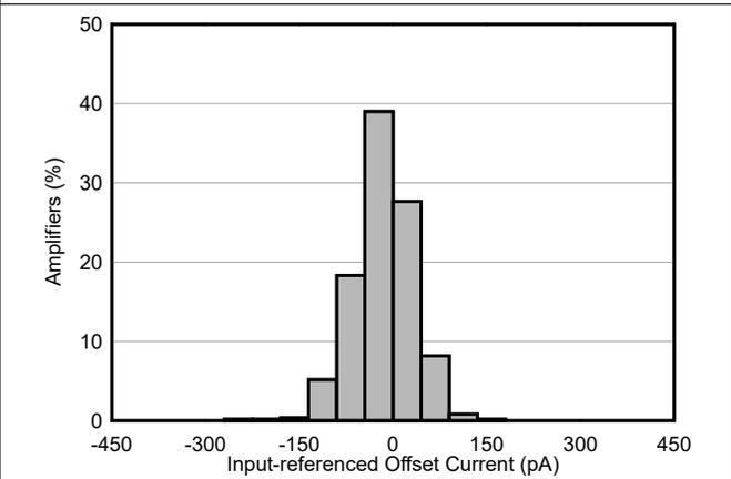
Figure 5-22. Input Offset Current Production Distribution
