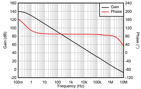
Figure 5-14. Open-Loop Gain and Phase vs Frequency
