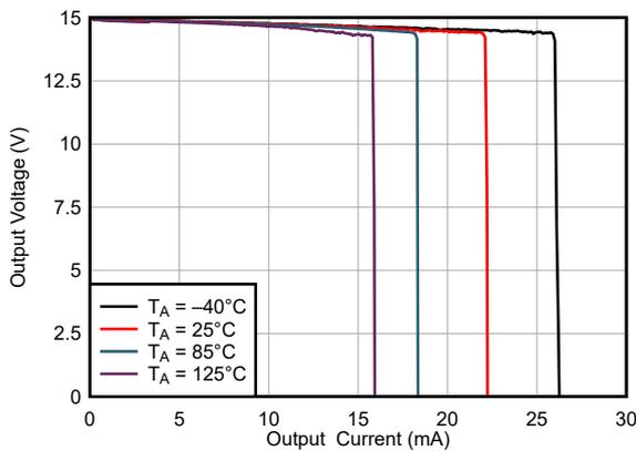
**Figure 5-29. Output Voltage Swing vs Output Sourcing Current**
