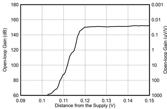
Figure 5-15. Open-Loop Gain vs Distance From Supply
