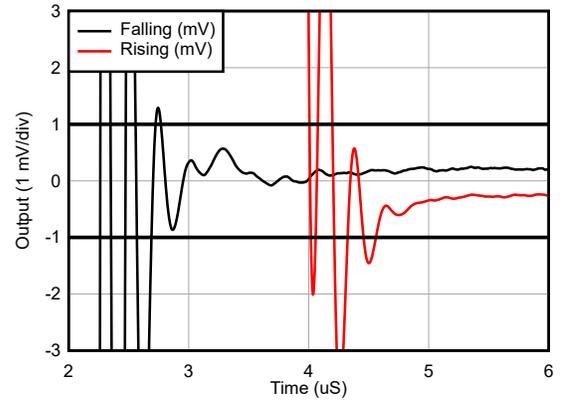
Figure 5-38. Settling Time
