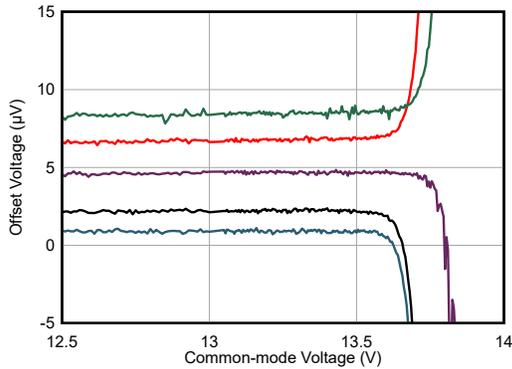
Figure 5-13. Offset Voltage vs  $V_{CM}$  at High Supply
