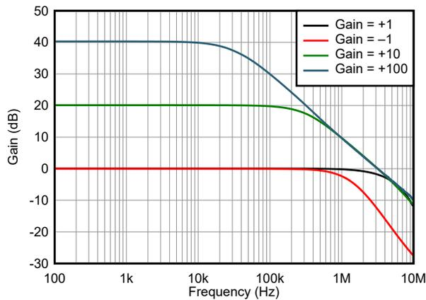
Figure 5-17. Closed-Loop Gain vs Frequency
