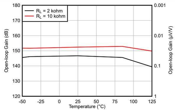
Figure 5-16. Open-Loop Gain vs Temperature
