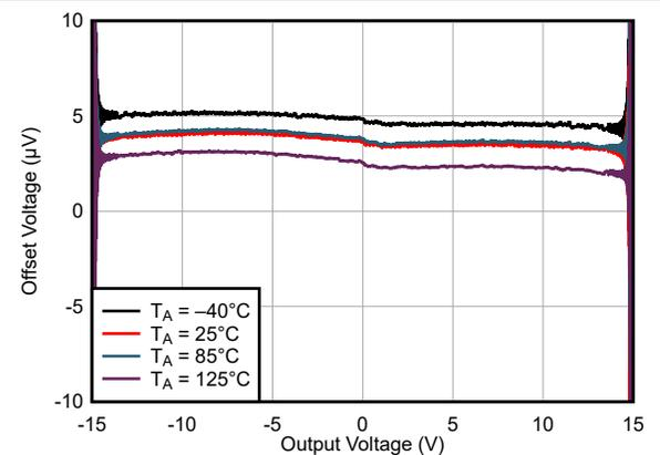
**Figure 5-6. Offset Voltage vs Output Voltage**
