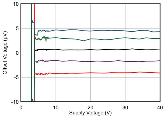
**Figure 5-7. Offset Voltage vs Power Supply Voltage**
