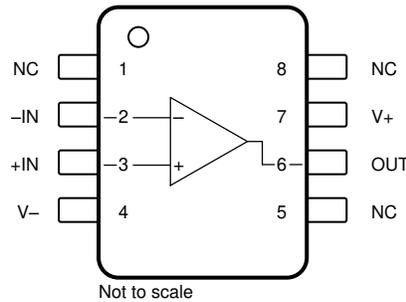
**Figure 4-1. OPA206: D Package, 8-Pin SOIC (Top View)**
