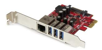
This PCIe USB 3.2 Gen 1 card couples your peripheral and network connections into a single, scalable solution.
