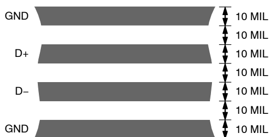
Figure 19. Arrangement of Signal Tracks
