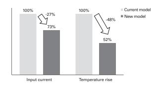
Fig. 4 Comparison of input current and temperature rise (SM2562C30B41)
