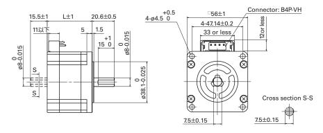
Fig. 2 Dimensions of the new model
