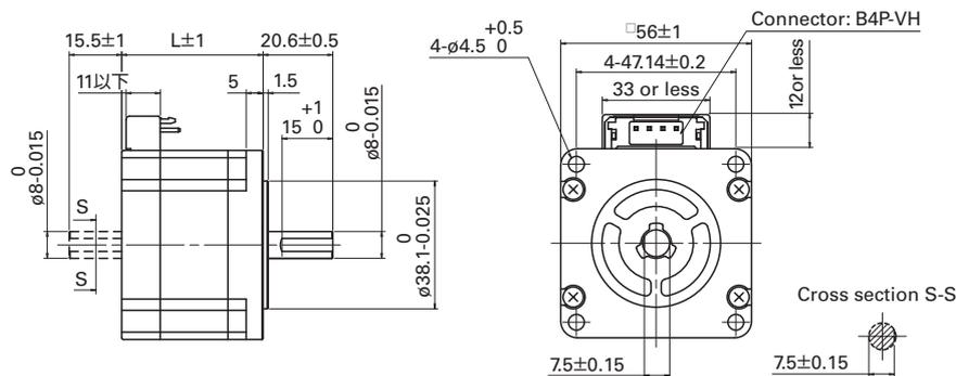
Fig. 2 Dimensions of the new model
