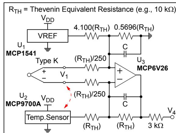
**FIGURE 4-16:** Thermocouple Sensor.
