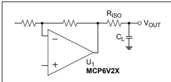
**FIGURE 4-7:** Output Resistor,  $R_{ISO}$ , Stabilizes Capacitive Loads.
