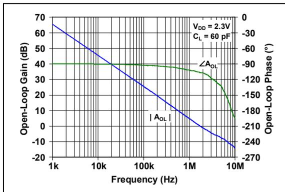
**FIGURE 2-26:** Open-Loop Gain vs. Frequency with  $V_{DD} = 2.3\text{V}$ .
