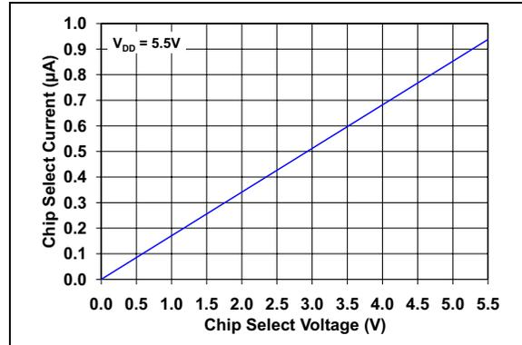
**FIGURE 2-54:** Chip Select Current vs. Chip Select Voltage.
