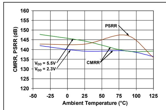
**FIGURE 2-12:** CMRR and PSRR vs. Ambient Temperature.
