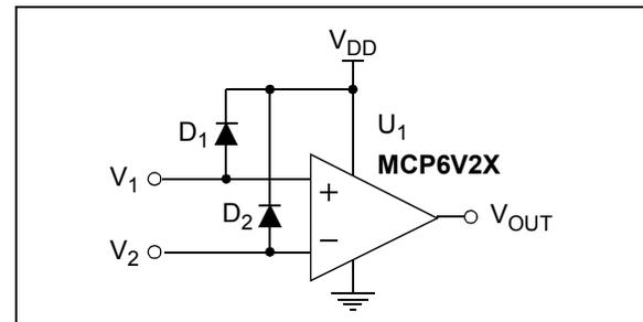
**FIGURE 4-5:** Protecting the Analog Inputs Against High Voltages.
