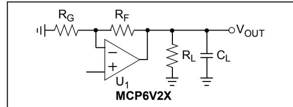
**FIGURE 4-9:** Output Load.
