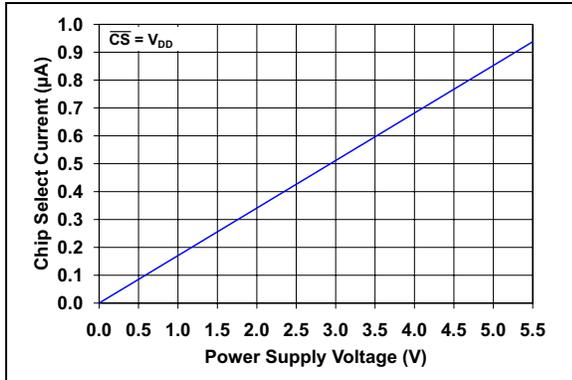
**FIGURE 2-51:** Chip Select Current vs. Power Supply Voltage.
