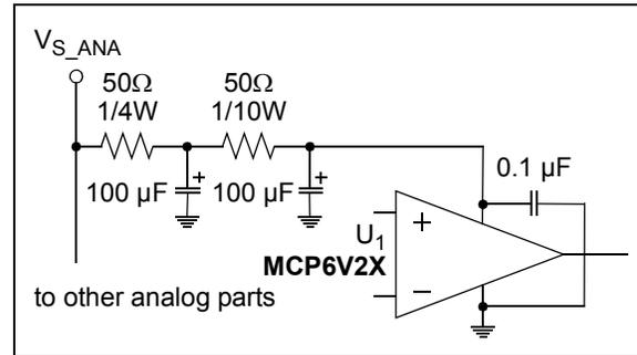
**FIGURE 4-11:** Additional Supply Filtering.
