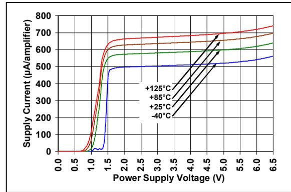
**FIGURE 2-22:** Supply Current vs. Power Supply Voltage.
