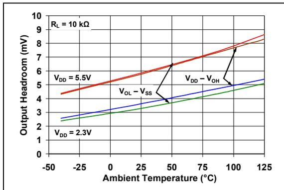
**FIGURE 2-20:** Output Voltage Headroom vs. Ambient Temperature.
