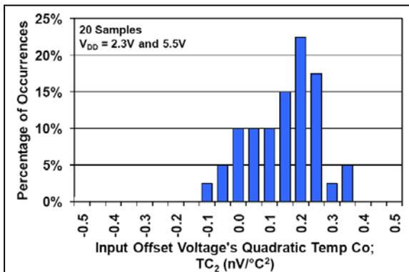
**FIGURE 2-3:** Input Offset Voltage Quadratic Temperature Coefficient.
