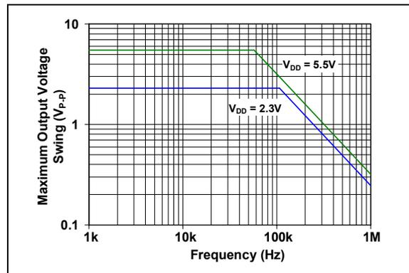
**FIGURE 2-34:** Maximum Output Voltage Swing vs. Frequency.
