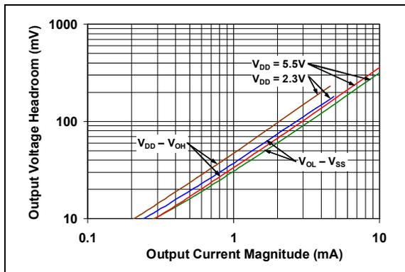
**FIGURE 2-19:** Output Voltage Headroom vs. Output Current.
