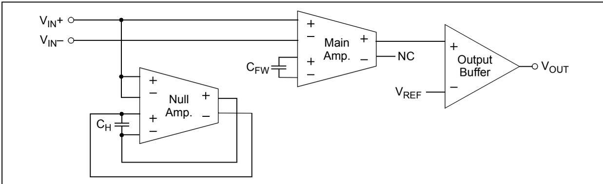
**FIGURE 4-3:** Auto-zeroing Mode of Operation ( $\phi_2$ ); Equivalent Diagram.
