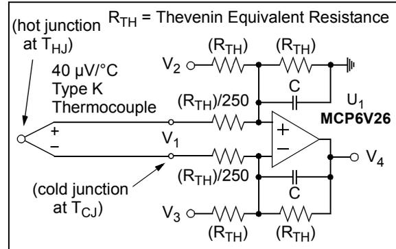
**FIGURE 4-15:** Thermocouple Sensor; Simplified Circuit.
