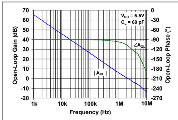
**FIGURE 2-27:** Open-Loop Gain vs. Frequency with  $V_{DD} = 5.5\text{V}$ .
