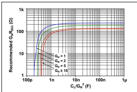
**FIGURE 4-8:** Recommended  $R_{ISO}$  values for Capacitive Loads.
