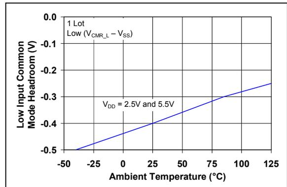
FIGURE 2-5: Low-Input Common-Mode Voltage Headroom vs. Ambient Temperature.
