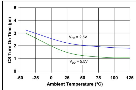
**FIGURE 2-45:**  $\overline{\text{CS}}$  Turn-On Time vs. Ambient Temperature.
