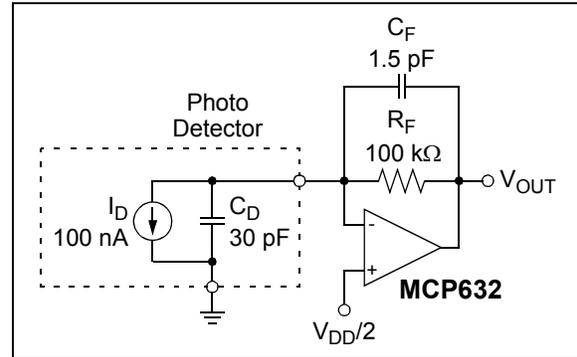
FIGURE 4-11: Transimpedance Amplifier for an Optical Detector.
