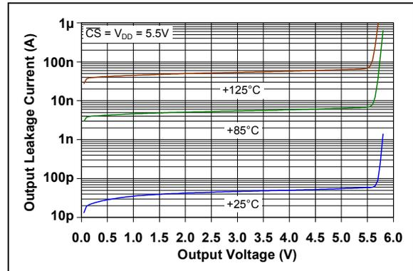
**FIGURE 2-48:** Output Leakage Current vs. Output Voltage.
