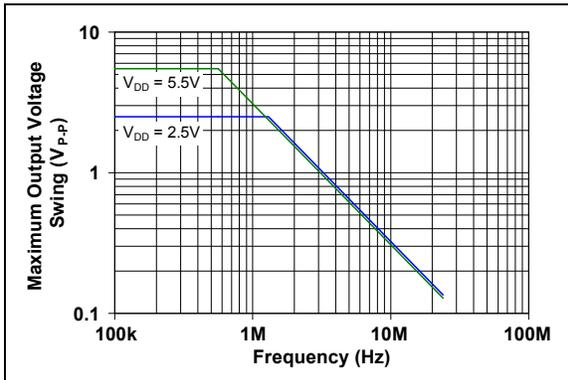
**FIGURE 2-40:** Maximum Output Voltage Swing vs. Frequency.
