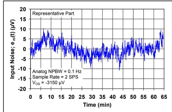
**FIGURE 2-32:** Input Noise vs. Time with 0.1 Hz Filter.
