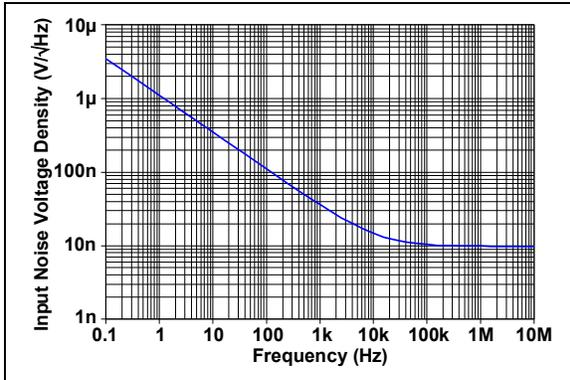
**FIGURE 2-29:** Input Noise Voltage Density vs. Frequency.
