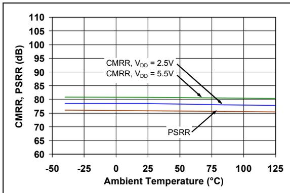
**FIGURE 2-9:** CMRR and PSRR vs. Ambient Temperature.
