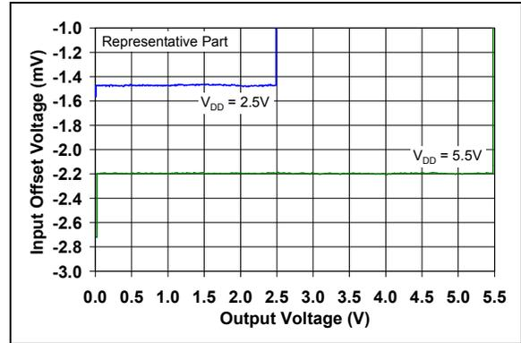
FIGURE 2-4: Input Offset Voltage vs. Output Voltage.
