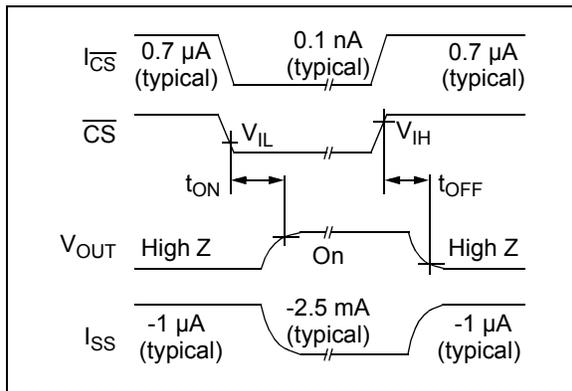
**FIGURE 1-1:** Timing Diagram.
