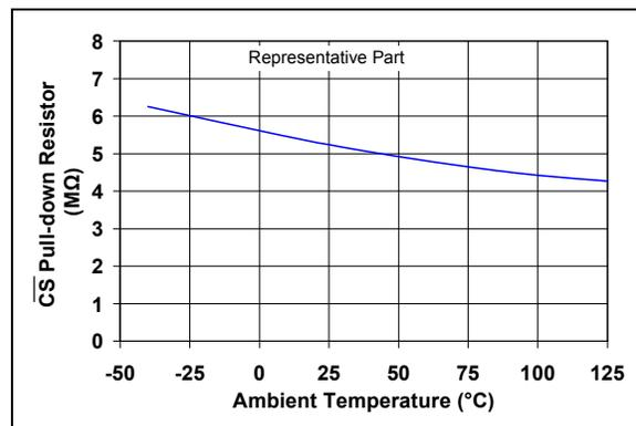
**FIGURE 2-46:**  $\overline{\text{CS}}$  Pull-down Resistor ( $R_{PD}$ ) vs. Ambient Temperature.
