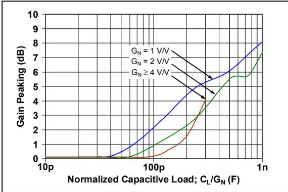
**FIGURE 2-27:** Gain Peaking vs. Normalized Capacitive Load.
