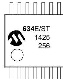
16-Lead QFN (4x4x0.9 mm) (MCP639)
