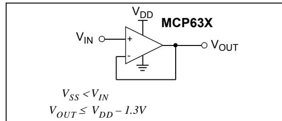
**FIGURE 4-3:** Unity-Gain Voltage Limitations for Linear Operation.
