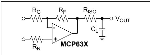
**FIGURE 4-6:** Output Resistor,  $R_{ISO}$ , Stabilizes Large Capacitive Loads.
