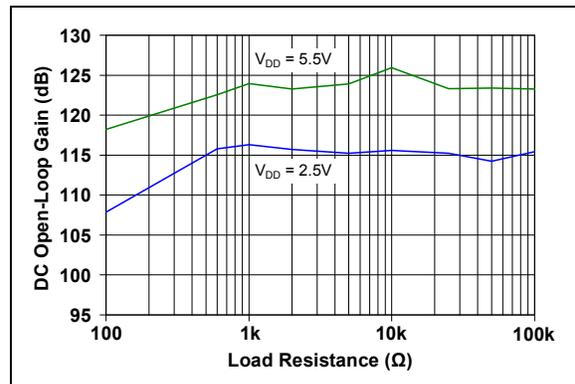
**FIGURE 2-11:** DC Open-Loop Gain vs. Load Resistance.
