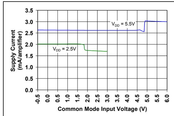
**FIGURE 2-20:** Supply Current vs. Common-Mode Input Voltage.
