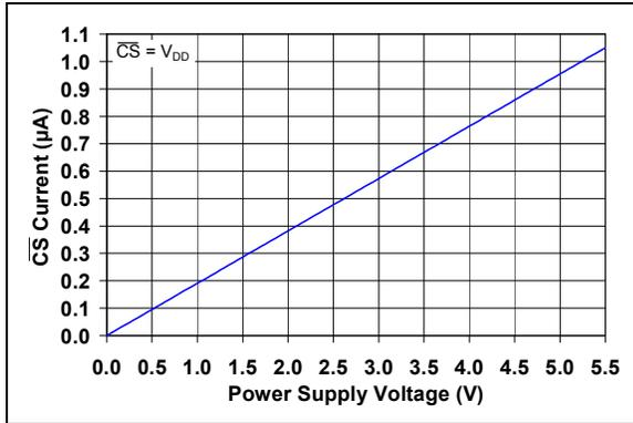
**FIGURE 2-41:**  $\overline{\text{CS}}$  Current vs. Power Supply Voltage.
