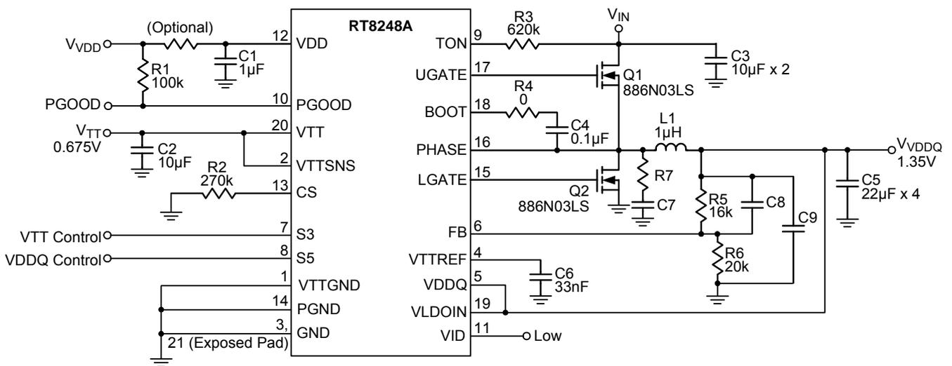
Figure 2. Typical Application Circuit with Pure MLCC Solution
