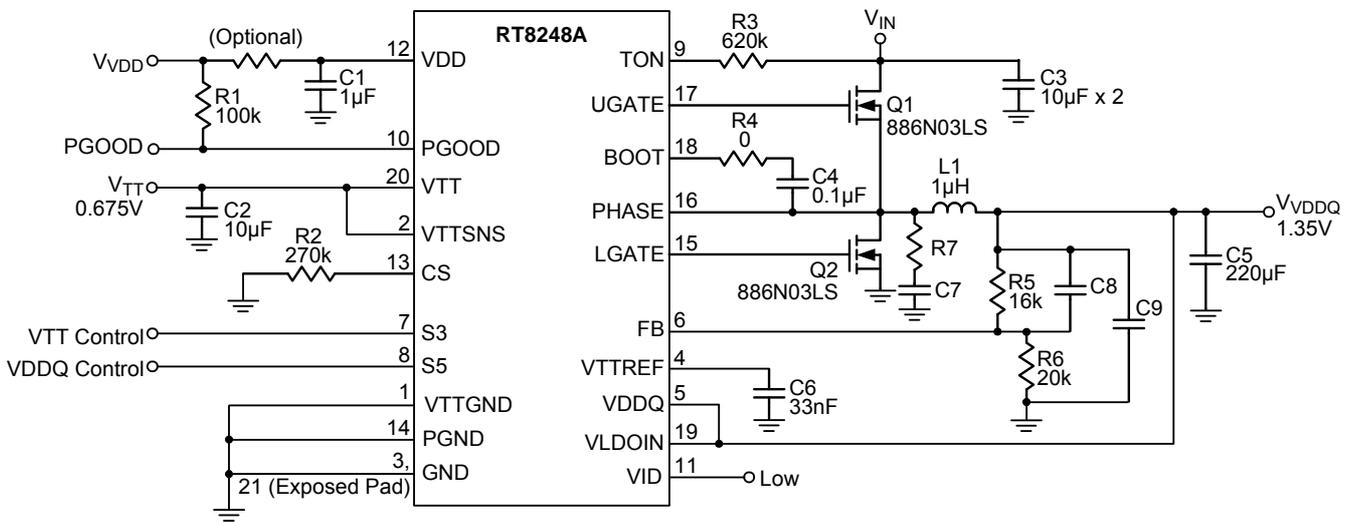
Figure 1. Typical Application Circuit with POSCAP Solution
