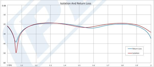
Click the following link (or enter part number in "SEARCH" on website) to obtain additional part information including price, inventory and certifications: High Power Isolator with 18 dB Isolation from 1 GHz to 2 GHz, 100 Watts and N Female PE83IR1001
