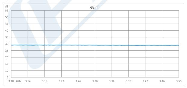
Click the following link (or enter part number in "SEARCH" on website) to obtain additional part information including price, inventory and certifications: 0.8 dB NF Input Protected Low Noise Amplifier, Operating from 3.1 GHz to 3.5 GHz with 28 dB Gain, 8 dBm P1dB and SMA PE15A63010
