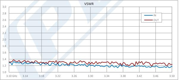
Click the following link (or enter part number in "SEARCH" on website) to obtain additional part information including price, inventory and certifications: 0.8 dB NF Input Protected Low Noise Amplifier, Operating from 3.1 GHz to 3.5 GHz with 28 dB Gain, 8 dBm P1dB and SMA PE15A63010
