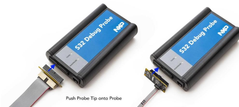
**Note:** Pin 1 is clearly marked on the gray ribbon cable by a red line down one side of the cable and a small triangle in the plastic socket.
