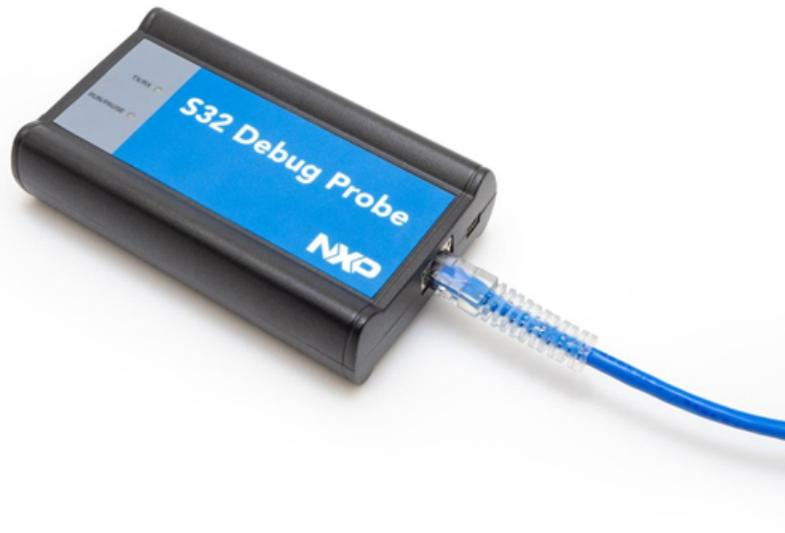
**Note:** When you configure the debugger for the hardware connection, you will need to specify the S32 Debug Probe IP address or hostname. The CCS findcc utility is used to search any probe on the local subnet. For more information, see [Using CCS to search for S32 Debug Probes](#) on page 27 topic.
