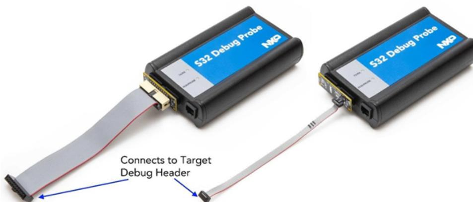
5. Gently (but firmly) press the connector onto the target system debug port header.
