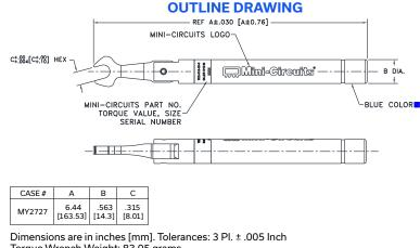
Torque Wrench Weight: 83.05 grams Torque Wrench + Box Weight: 175 grams
