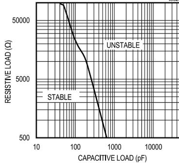
STABILITY vs. CAPACITIVE LOAD AND ISOLATION RESISTOR
