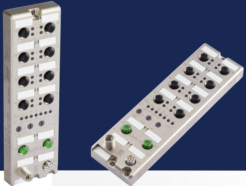
The new, innovative LioN-X Digital I/O Modules offer highest adaptability with five Industrial Ethernet and four IIoT Protocols onboard while also ensuring advanced security. Four different Input/ Output variants provide maximum flexibility for your application.
