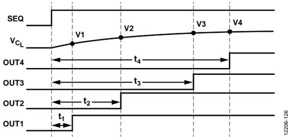
Figure 26. Programmable Sequencing Control Circuit Timing Diagram
