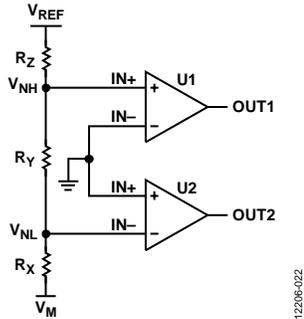
Figure 23. Negative Undervoltage/Overvoltage Monitoring Configuration
