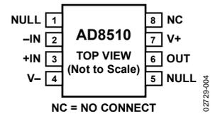
Figure 2. 8-Lead SOIC\_N (R Suffix)
