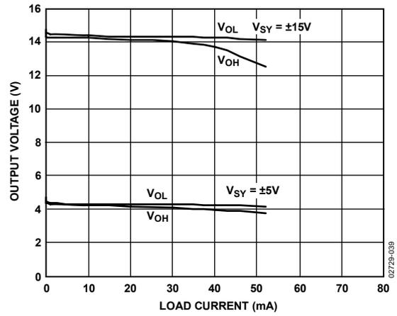
Figure 39. AD8513 Output Voltage vs. Load Current
