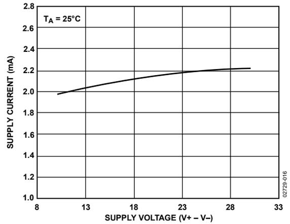
Figure 16. AD8510 Supply Current vs. Supply Voltage
