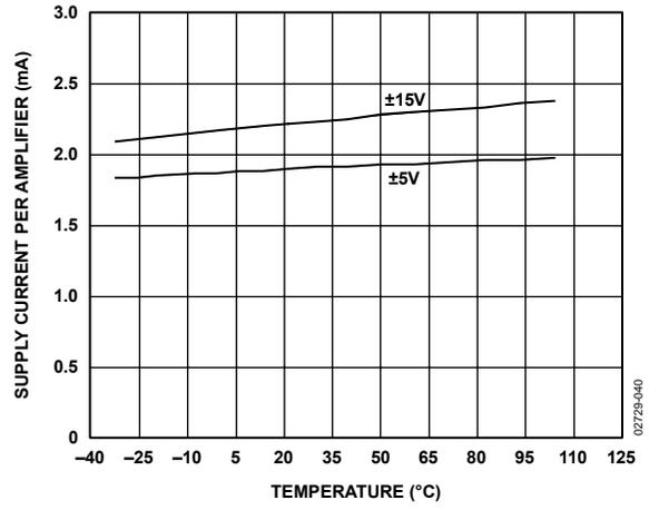
Figure 40. AD8513 Supply Current per Amplifier vs. Temperature
