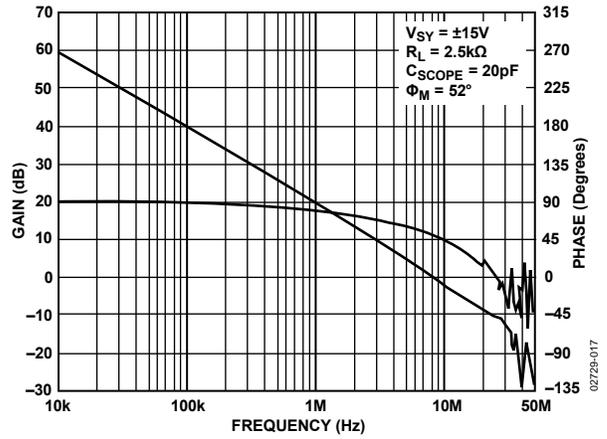
Figure 17. Open-Loop Gain and Phase vs. Frequency
