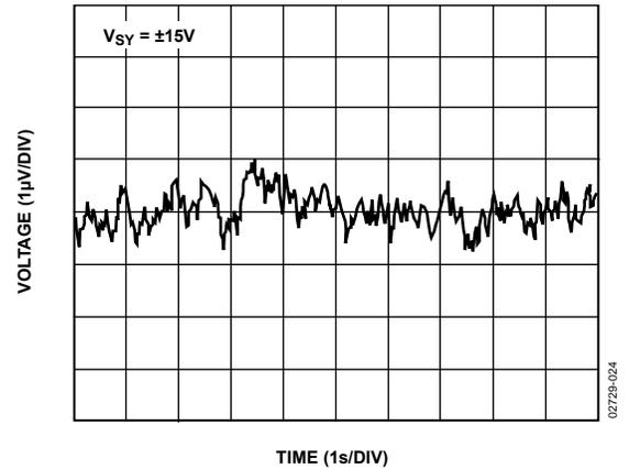
Figure 24. 0.1 Hz to 10 Hz Input Voltage Noise
