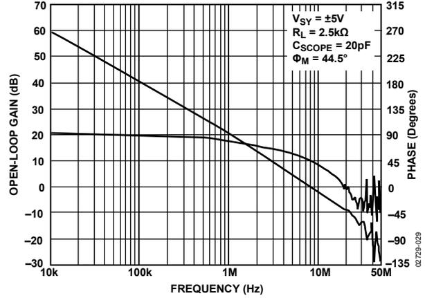
Figure 29. Open-Loop Gain and Phase vs. Frequency
