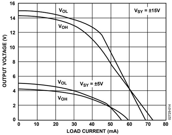
Figure 14. AD8510/AD8512 Output Voltage vs. Load Current
