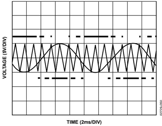
Figure 55. Pulse-Width Modulation
