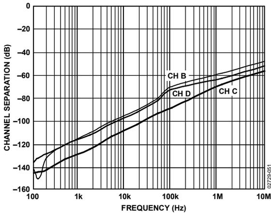
Figure 57. Channel Separation
