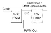
Figure 2. TS2000 Haptics Block Diagram: Two Digital Blocks Configuration, Interrupt and Polled Update Method
