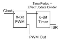
Figure 3. TS2000 Haptics Block Diagram. One Digital Block Configuration, Direct Update Method Option
