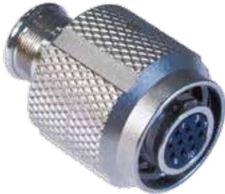
**Series 805 Environmental Plugs:** feature two shell styles including Integral banding porch version for direct shield attachment using Band-Master ATS® termination system, or accessory thread version for attaching a connector backshell or strain relief. EMI ground spring achieves low shell-to-shell resistance. This nickel-plated beryllium copper spring enables the
