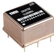
This TSE module contains an SC-cut ovenized crystal oscillator combined with a temperature sensor and internal EEPROM. The internal EEPROM contains polynomial coefficients calculated through a curve fitting of the frequency versus temperature data set. The module's I2C pins provide communication access to the temp sensor and stored data in the EEPROM available to be read directly by the compensating ICs or compensating modules when the pins are connected according to documented specifications.
