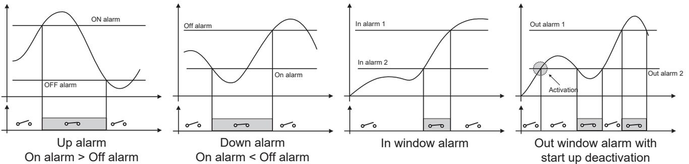
**Note:** any alarm working mode can be linked to the "start up deactivation" function which disables only the first alarm after power on of the transducer.
