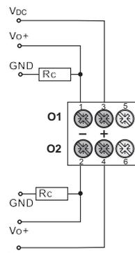
Open collector outputs: The load resistance ( $R_c$ ) must be calculated so that the closed contact current is lower than 100mA; the VDC voltage must be lower than or equal to 30V. VDC: power supply voltage (external). Vo+: positive output contact (open collector transistor). GND: ground output contact (open collector transistor).
