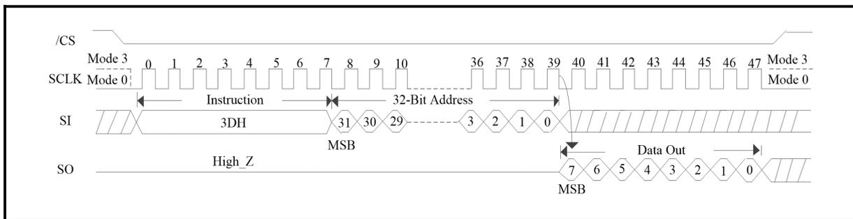
**Figure 183. Read DPB Status (QPI Mode/3-Byte Address Mode)**
