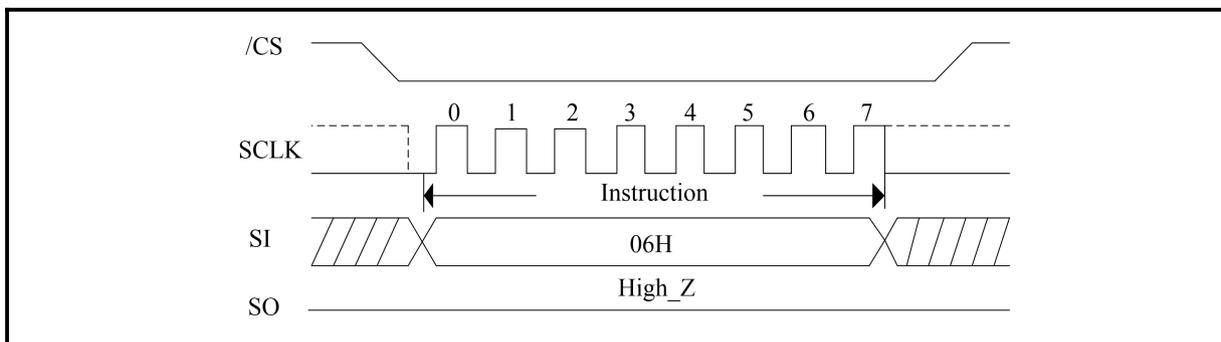
**Figure 12. Write Enable Sequence Diagram (QPI Mode)**
