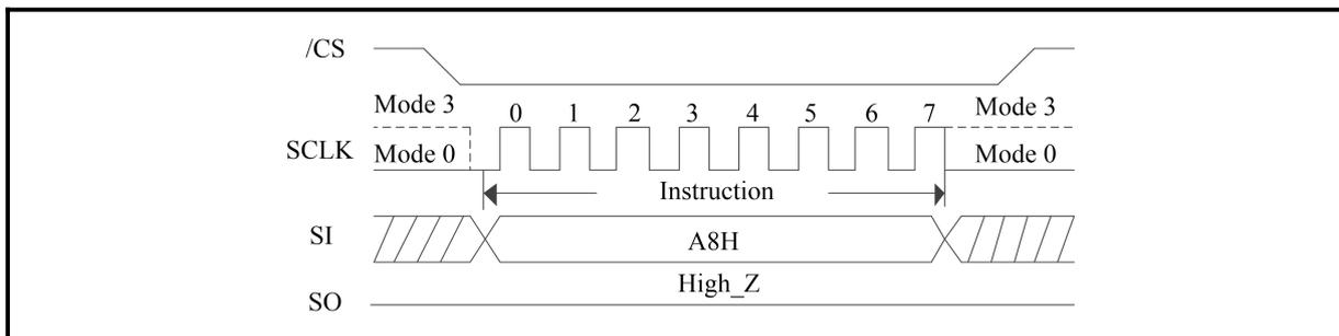
**Figure 196. Unprotect Solid Protect Bit Set (QPI Mode)**
