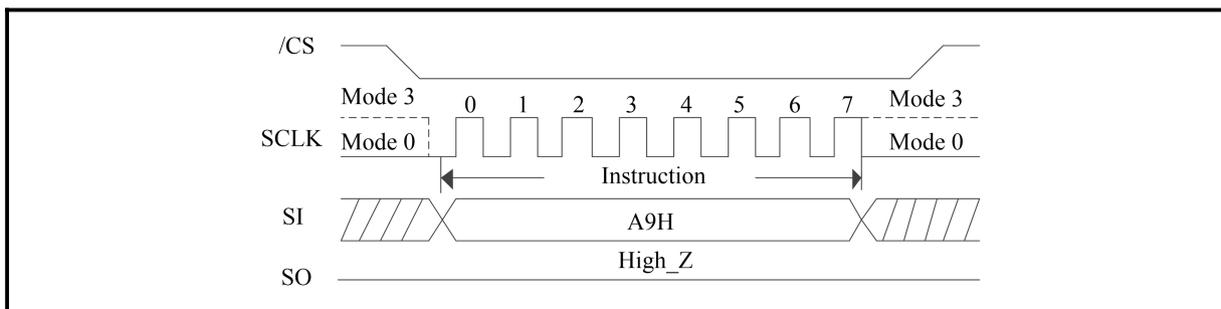
**Figure 198. Unprotect Solid Protect Bit Clear (QPI Mode)**
