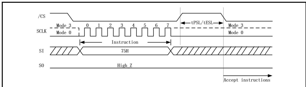
**Figure 160. Program/Erase Suspend Instruction Sequence (QPI Mode)**
