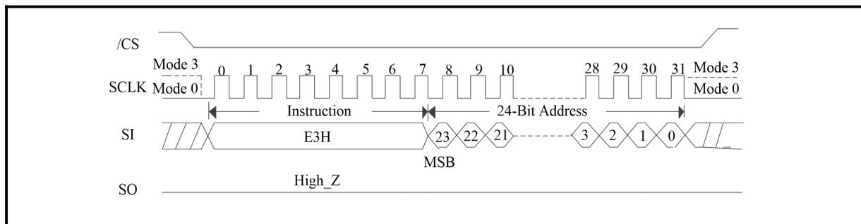
**Figure 176. SPB Program (SPI Mode/4-Byte Address Mode)**
