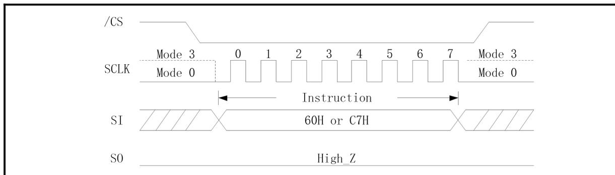
**Figure 158. Chip Erase Sequence Diagram (QPI Mode)**
