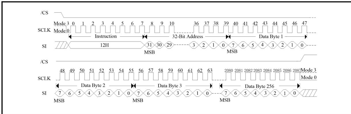
**Figure 135. Page Program with 4-Byte Address (QPI Mode)**
