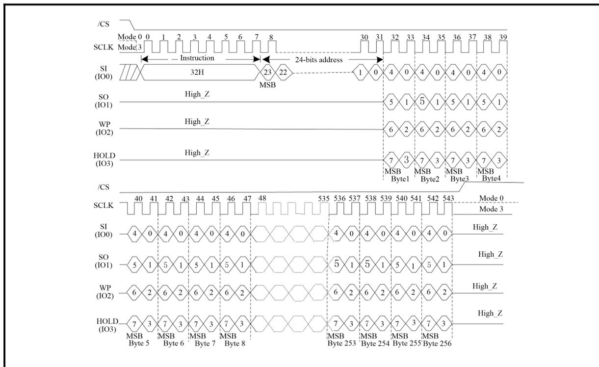
**Figure 137. Quad Page Program Sequence Diagram (SPI Mode only/4-Byte Address Mode)**
