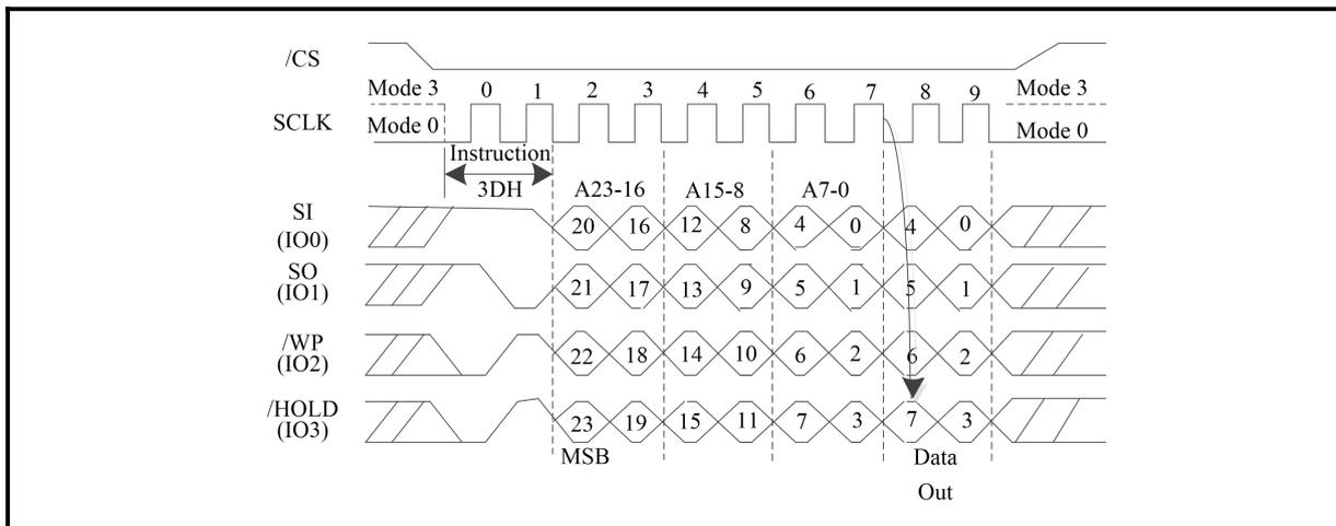
**Figure 184. Read DPB Status (QPI Mode/4-Byte Address Mode)**
