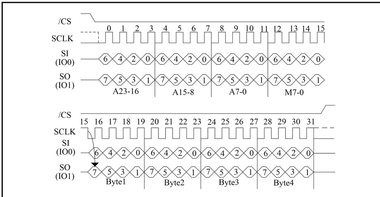
**Figure 56. Dual I/O Fast Read Sequence Diagram (SPI Mode/4-Byte Address Mode; Previous instruction set (M5-4) =(1,0))**
