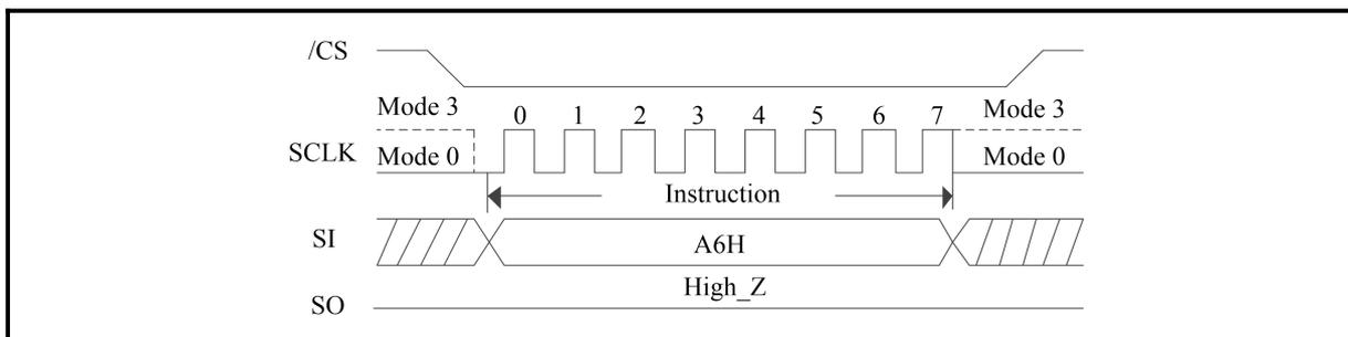
**Figure 168. SPB Lock Bit Clear (QPI Mode)**
