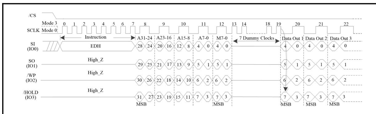
**Figure 73. DTR Fast Read Quad I/O (SPI Mode/3-Byte Address Mode; Initial instruction or previous (M5-4=(1,0)))**
