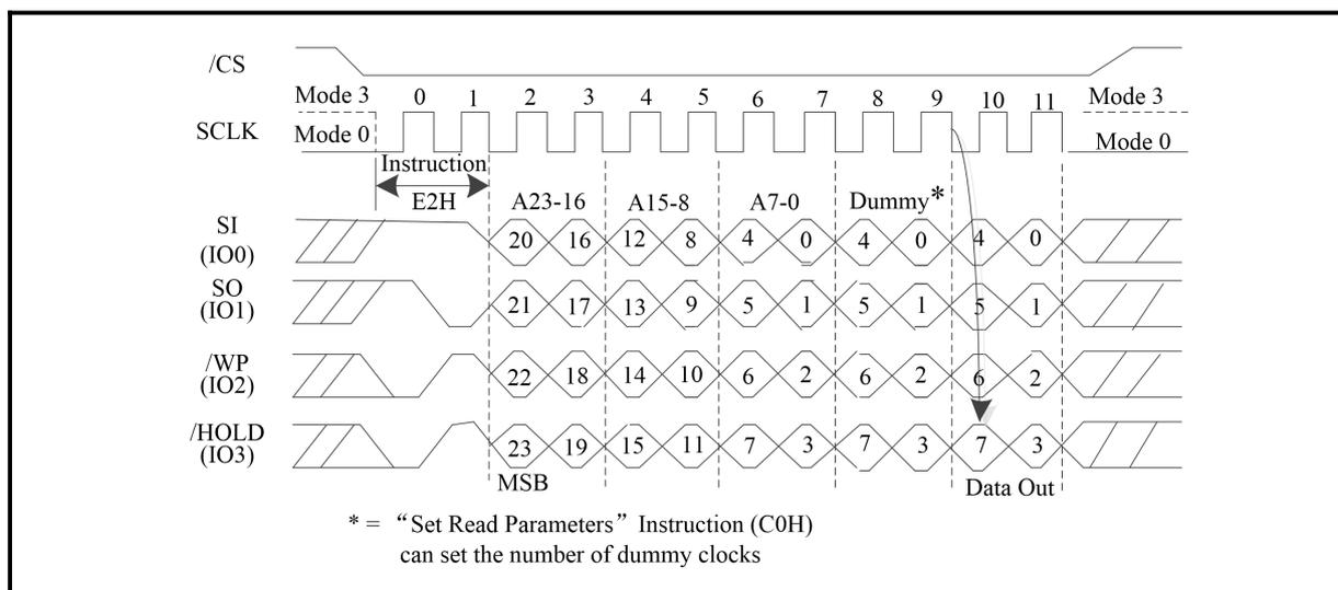
**Figure 174. Read SPB Status (QPI Mode/4-Byte Address Mode)**
