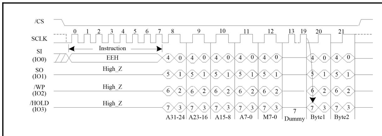
**Figure 84. DTR Quad I/O Fast Read with 4- Byte Address (SPI Mode; Initial instruction or previous M5-4=10)**
