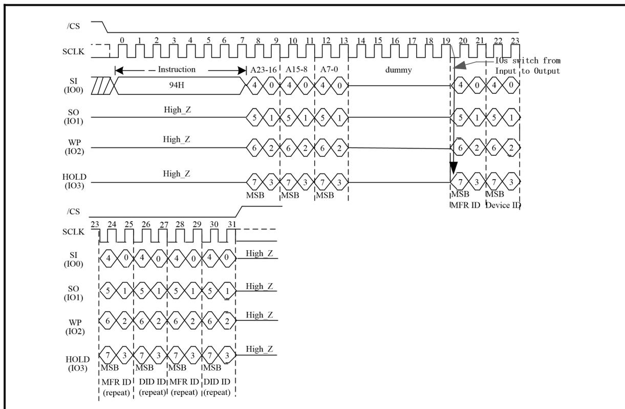
**Figure 103. Quad I/O Read Manufacture ID/ Device ID Sequence Diagram (SPI Mode/3-Byte Address Mode)**
