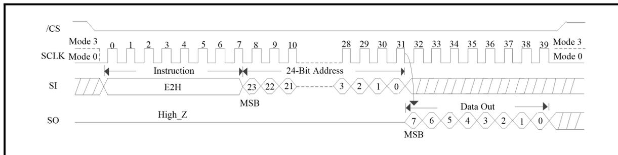
**Figure 172. Read SPB Status (SPI Mode/4-Byte Address Mode)**
