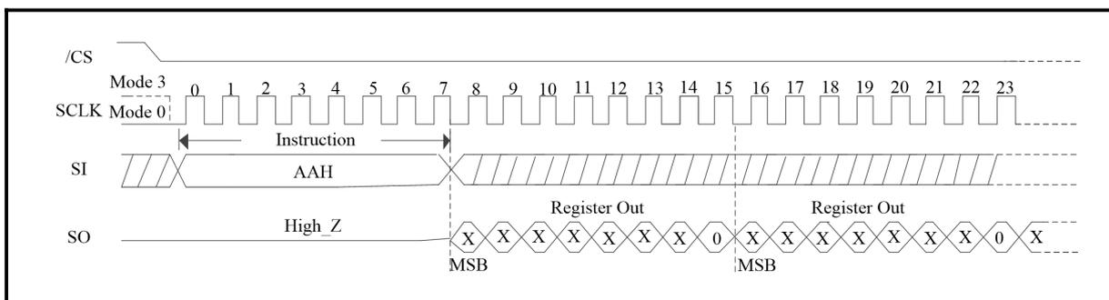
**Figure 194. Read Unprotect Solid Protect Bit (QPI Mode)**
