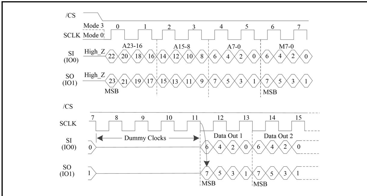
**Figure 60. DTR Fast Read Dual I/O (SPI Mode only/4-Byte Address Mode; Previous instruction set M5-4=10)**
