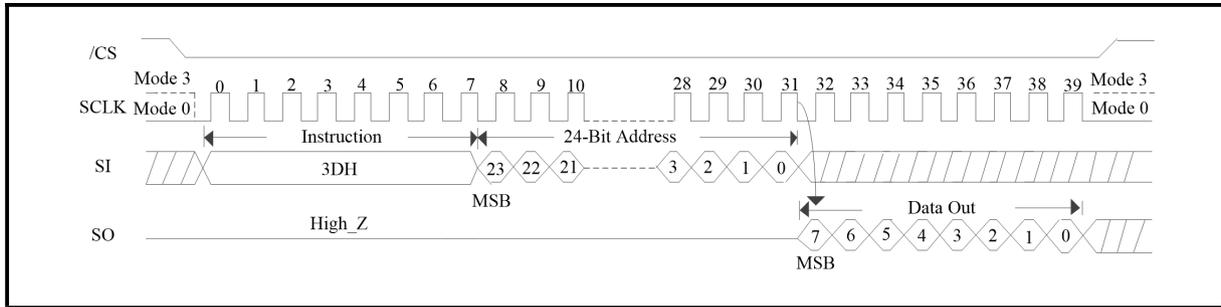
**Figure 182. Read DPB Status (SPI Mode/4-Byte Address Mode)**
