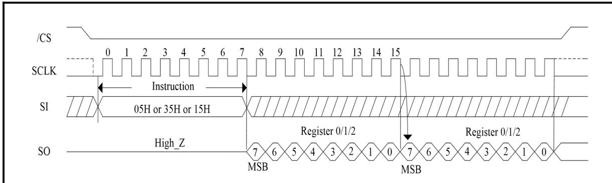
**Figure 18. Read Status Register Sequence Diagram (QPI Mode)**
