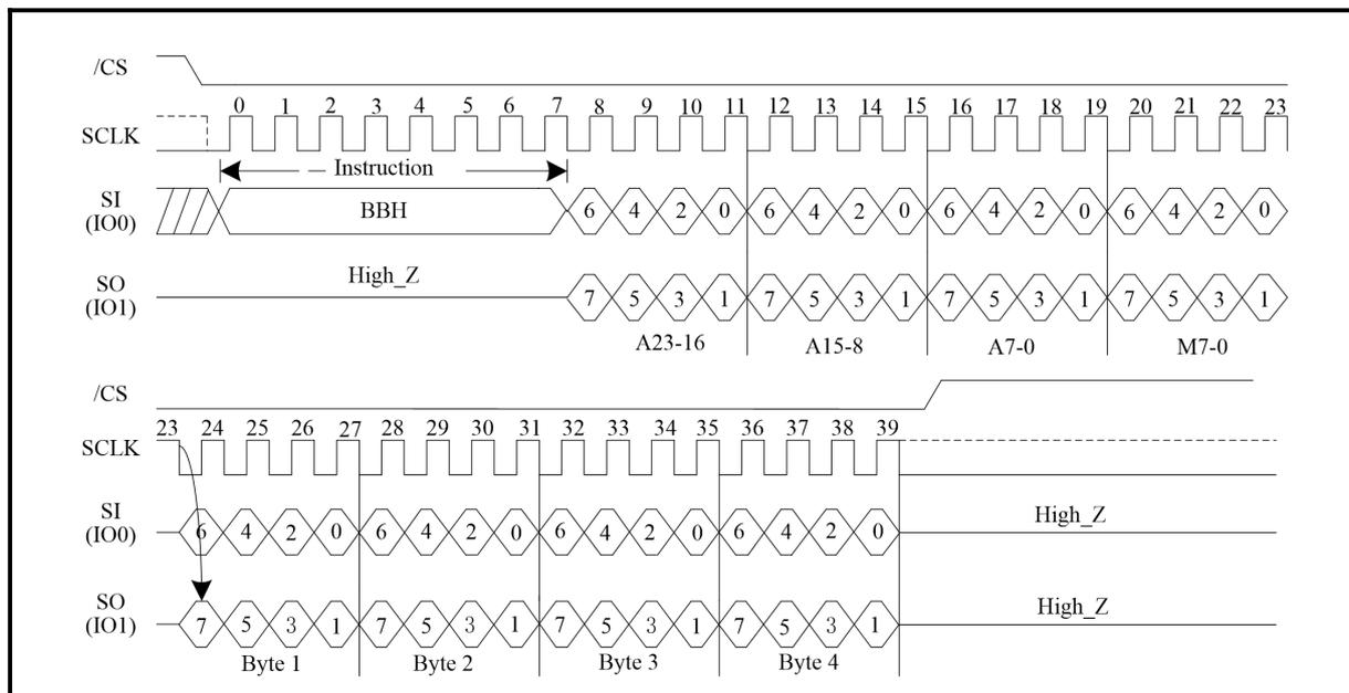
**Figure 54. Dual I/O Fast Read Sequence Diagram (SPI Mode/4-Byte Address Mode; Initial instruction or previous (M5-4)≠(1,0))**
