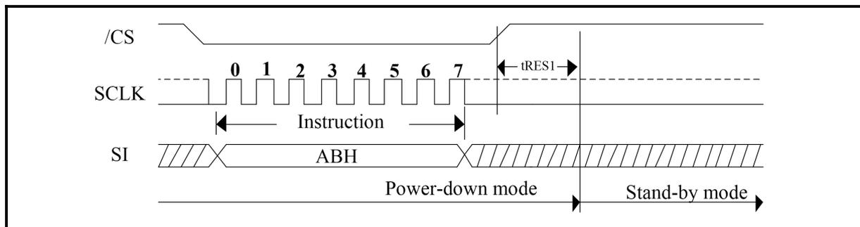
**Figure 113. Release Power-Down Sequence Diagram (QPI Mode)**
