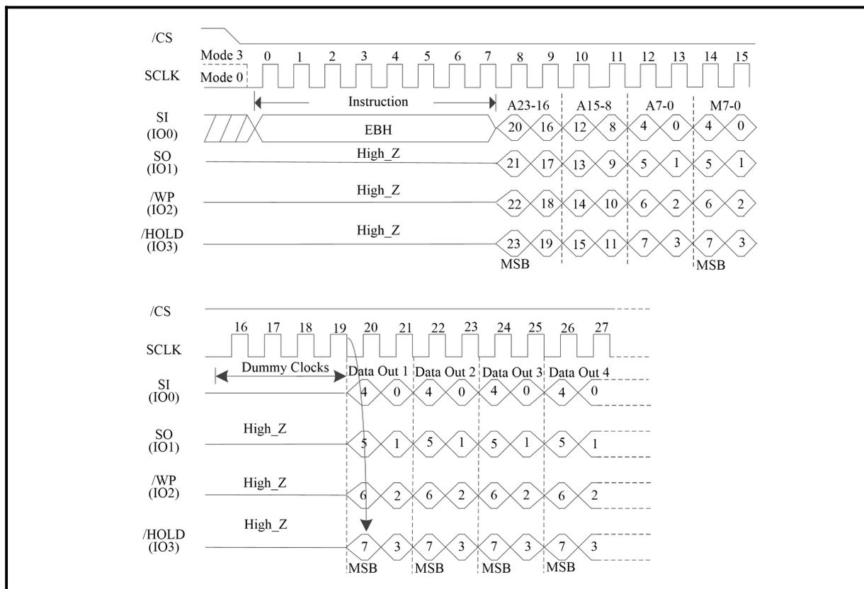
**Figure 64. Quad I/O Fast Read Sequence Diagram (SPI Mode/4-Byte Address Mode; Initial instruction or previous (M5-4≠(1,0)))**
