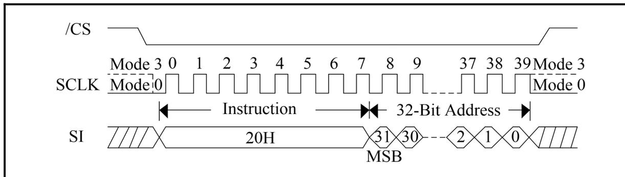
**Figure 141. Sector Erase Sequence Diagram (QPI Mode/3-Byte Address Mode)**
