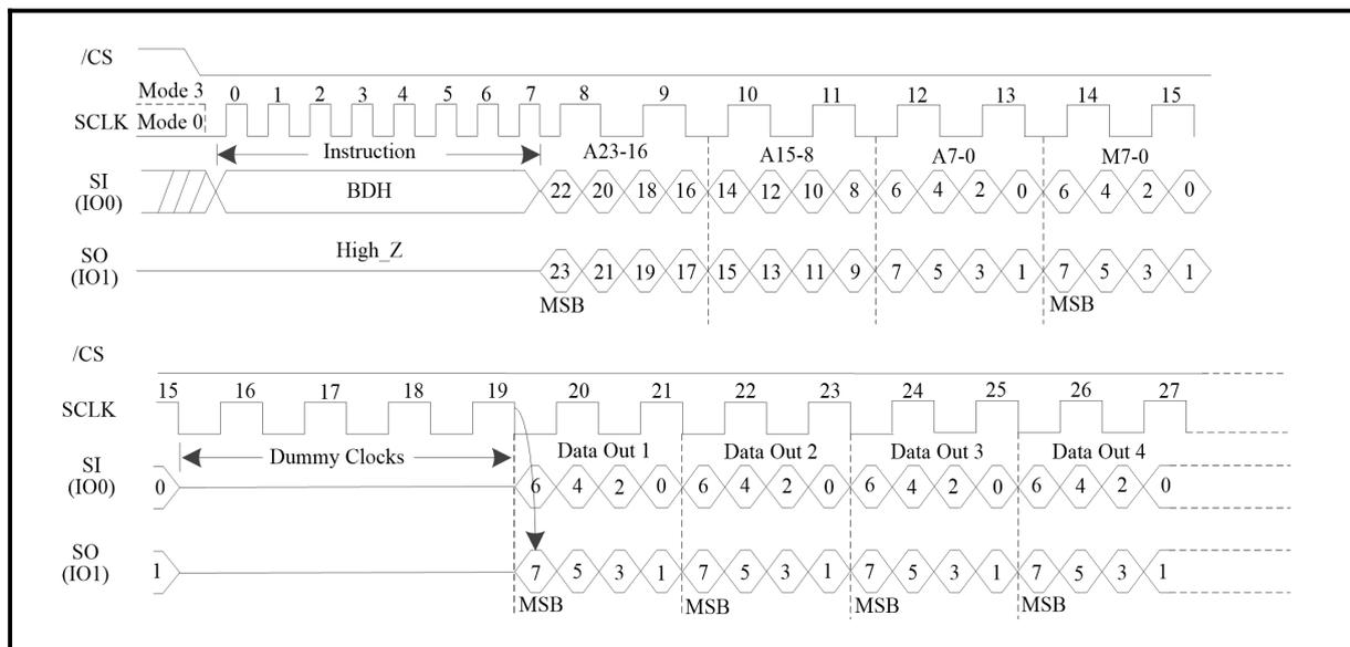
**Figure 58. DTR Fast Read Dual I/O (SPI Mode only/4-Byte Address Mode; Initial instruction or previous M5-4≠10)**
