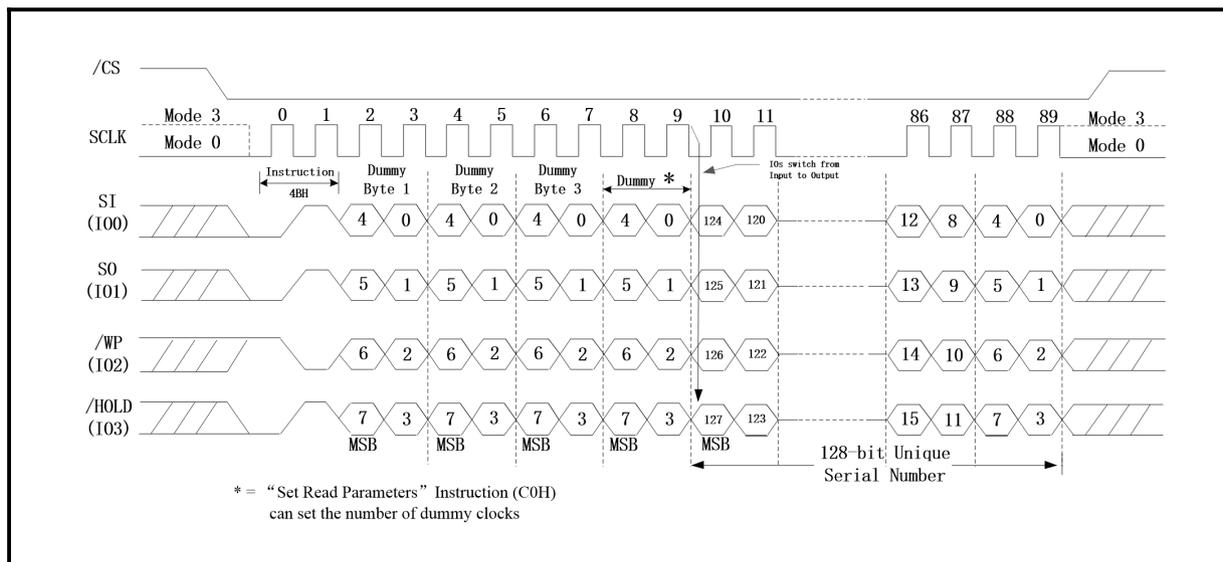
**Figure 109. Read Unique ID Sequence Diagram (QPI Mode/4-Byte Address Mode)**
