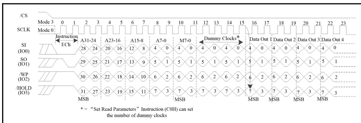
**Figure 82. Fast Read Quad I/O with 4-Byte Address (QPI Mode; Initial instruction or previous M5-4=10)**
