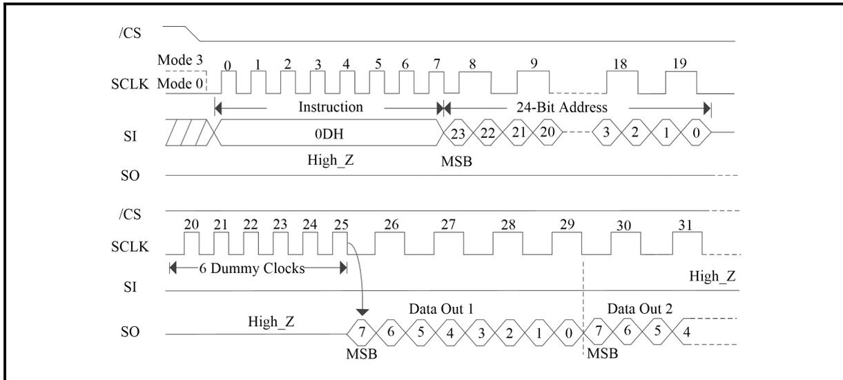
**Figure 43. DTR Fast Read (SPI Mode/4-Byte Address Mode)**
