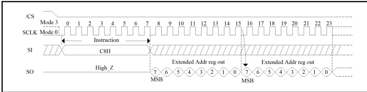
**Figure 24. Read Extended Address Register (QPI Mode)**
