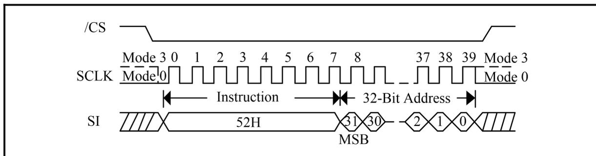
**Figure 147. 32KB Block Erase Sequence Diagram (QPI Mode/3-Byte Address Mode)**
