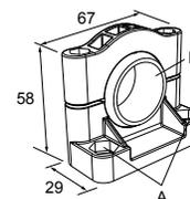
**Hole center spacing:** A=ø 50.8
