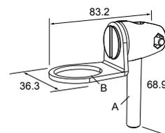
**Bolt thread:** SMB30FA, A= 3/8 - 16 x 2 in; SMB30FAM10, A= M10 - 1.5 x 50
