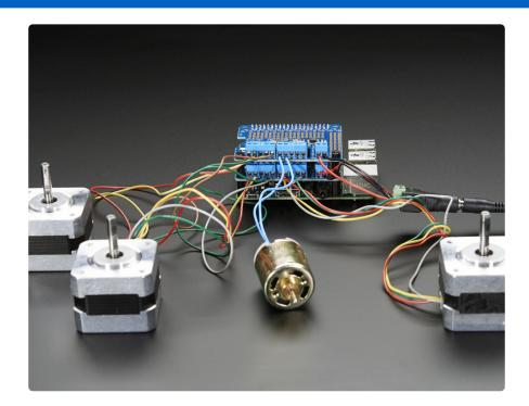
If connecting the Hat off-the Pi via jumpers, you will need to connect GND and 3.3v in addition to SDA and SCL.
