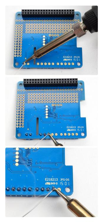
Flip over the board and solder in all of the terminal block pins
