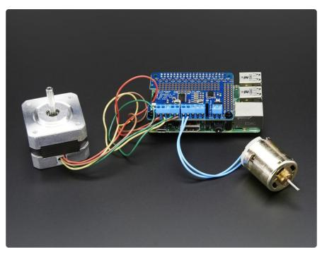
Let your robotic dreams come true with the new DC+Stepper Motor HAT from Adafruit. This Raspberry Pi add-on is perfect for any motion project as it can drive up to 4 DC or 2 Stepper motors with full PWM speed control.
