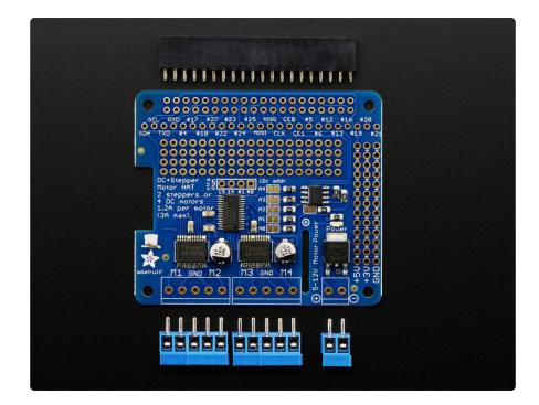
Comes with an assembled & tested HAT, terminal blocks, and 2x20 plain header. Some soldering is required to assemble the headers on. <u>Stacking header not</u> included, but we sell them in the shop so if you want to stack HATs, please pick one up at the same time. (http://adafru.it/2223)
