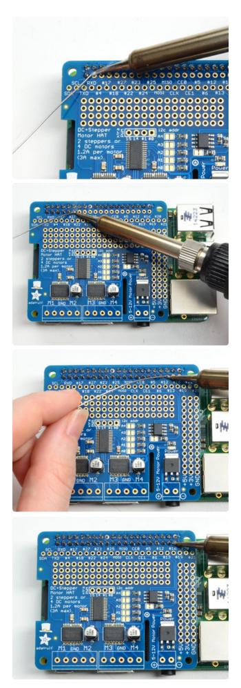
Flip the board around and solder all the connections for the other half of the 2x20 header
