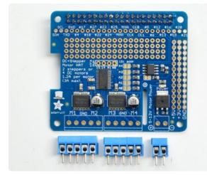
Now grab the 3.5mm-spaced terminal blocks. These will let you quickly connect up your motor and power supply using only a screw driver
