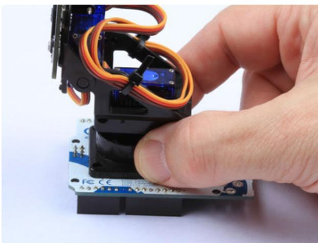
Position the camera as shown on the bottom of the Leonardo and press firmly to attach.
