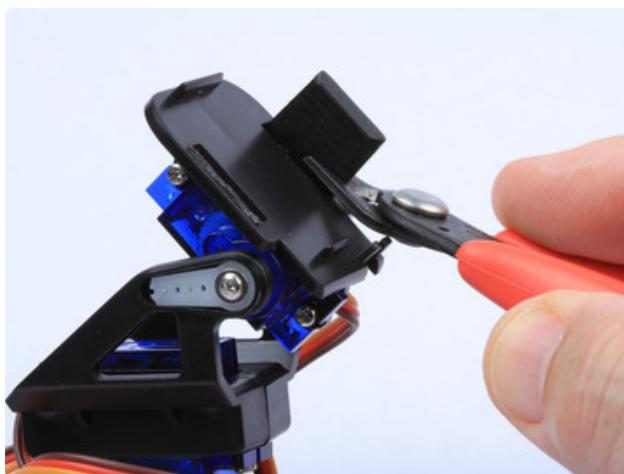
The bracket is made of a fairly soft nylon, so these are easily removed with a pair of wire cutters.
