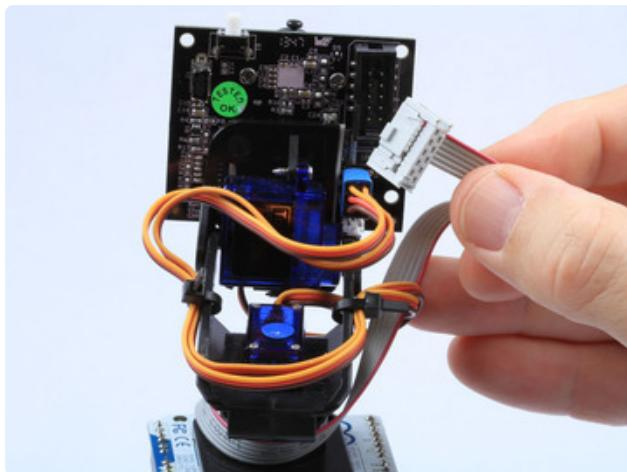
Attach the 8-pin end to the back of the Pixy. This connection is keyed, so there is only one way you can plug it in.
