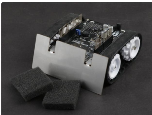
Using a piece of the packing foam from the Seeeduino kit, cut two small squares roughly 1.5" x 1.5" (3.5cm x 3.5cm) - These dimensions are not super critical!
