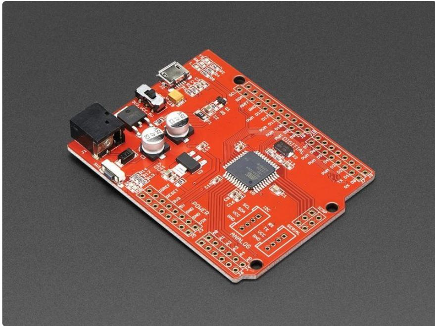
There is one little problem though. The Zumo chassis has a couple of unfortunately placed capacitors that interfere with the DC jack and capacitors on the Seeeduino.
