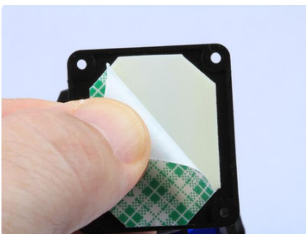
Cut a piece of foam tape to fit in the recess in the bottom of the pan/tilt base. (If you are using narrower tape, you can use multiple pieces.)
