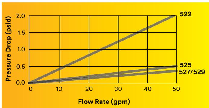
**Pressure Drop:** 3M™ 500 Series High Performance Filter Bags have low initial pressure drop ( $\Delta P$ ) in water as the chart indicates. The chart includes the pressure drop of a typical single vessel to assist filter system sizing.
