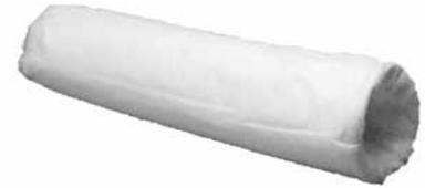
The 3M™ 500 series multi-layer, high efficiency filter bags are designed for use in fluid applications with high contaminant removal requirements. The bags utilize 3M polypropylene microfiber media. In addition to providing for high particle removal efficiency, the media also has a high capacity for trace oil removal. 3M 500 Series bags are offered in a Size #2 configuration in four micron grades; 2.5, 5.0, 15, and 48µm (at 99% Particle Removal Efficiency).
